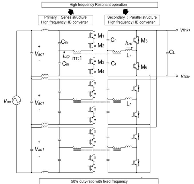
Fig. 1. Bidirectional high-frequency ac/dc converter.
