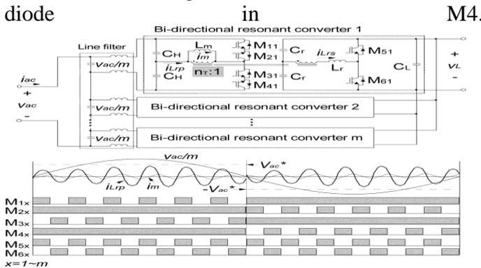
Fig. 2 AC/DC Resonant Converter and Switching Scheme.
