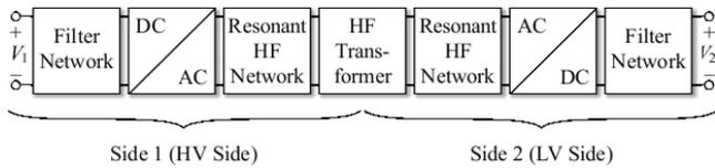
Fig 4: The different components required for an isolated, bidirectional DC-DC converter
