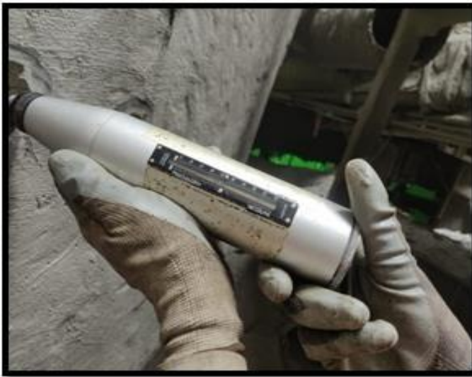
Fig No.1: - Rebound Hammer Test
