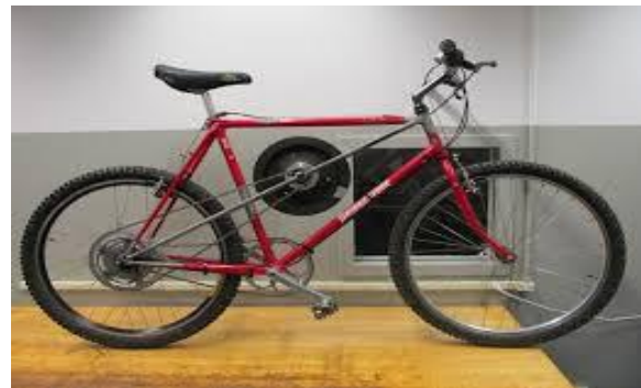
Fig1: Kinetic Energy Storage Mechanism In Bicycle
