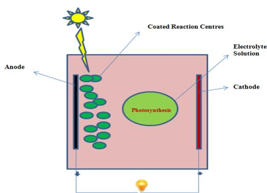
Fig. 1. Model of a Basic Bio Solar Cell
