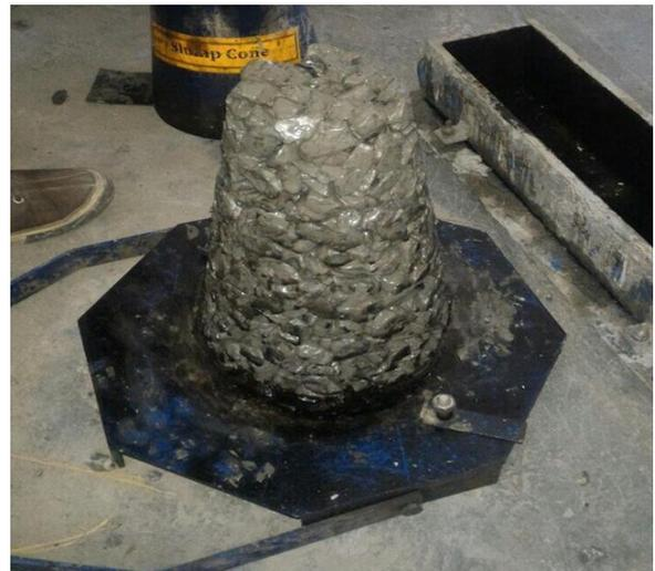
Fig. 1. Slump Test on concrete
