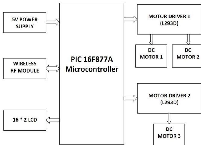
(Fig. B) Block Diagram of Robot ARM Control Unit
