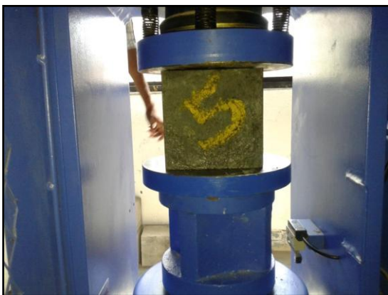
Fig. 3. Testing of 5% Replaced Concrete Cubes in compression testing machine
