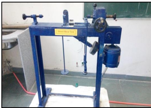
Fig. 2. Apparatus of Direct Shear Test
