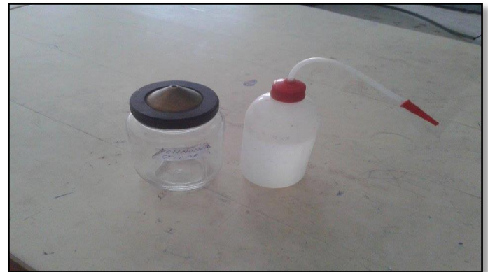
Fig. 1. Specific Gravity by Pycnometer method
