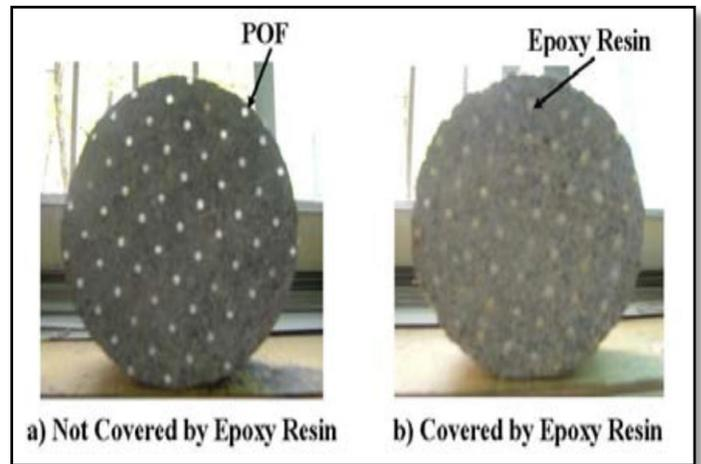
Fig. 4. Cylindrical concrete specimens for impermeability
