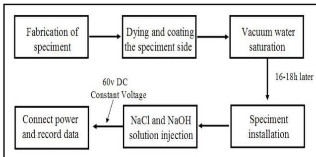
Fig. 7. Procedure of chloride diffusion coefficient test
